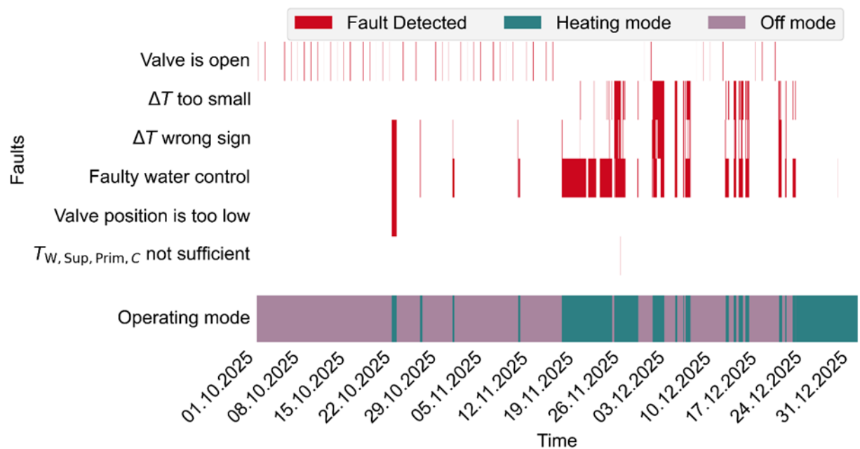
Figure 53: Heatmap of all fault types of the preheater occurred from the 01.10.2025 to the 31.12.2025 and operating mode of preheater. To facilitate visualization, data is aggregated into 1-
